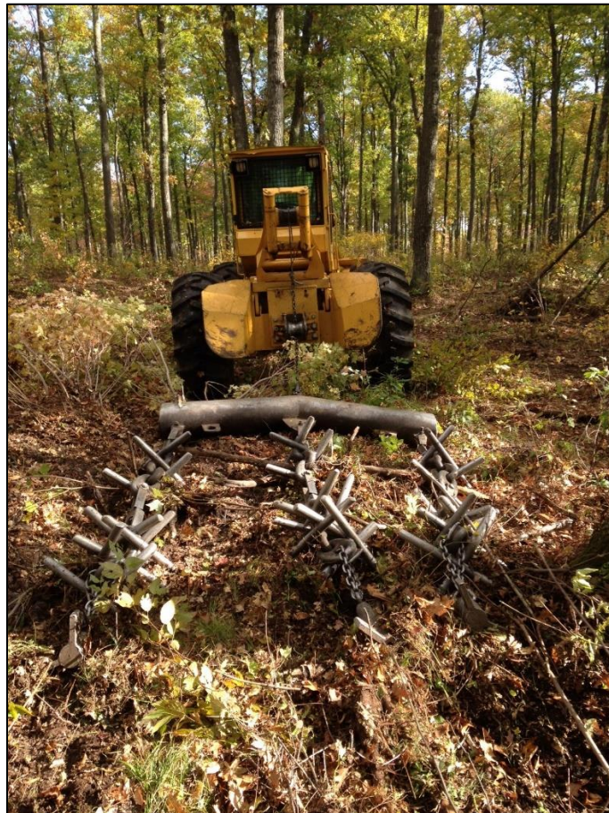
Anchor Chains Used For Understory Oak Scarification
