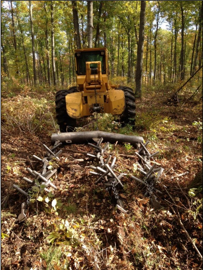
Anchor Chains Used For Understory Oak Scarification
