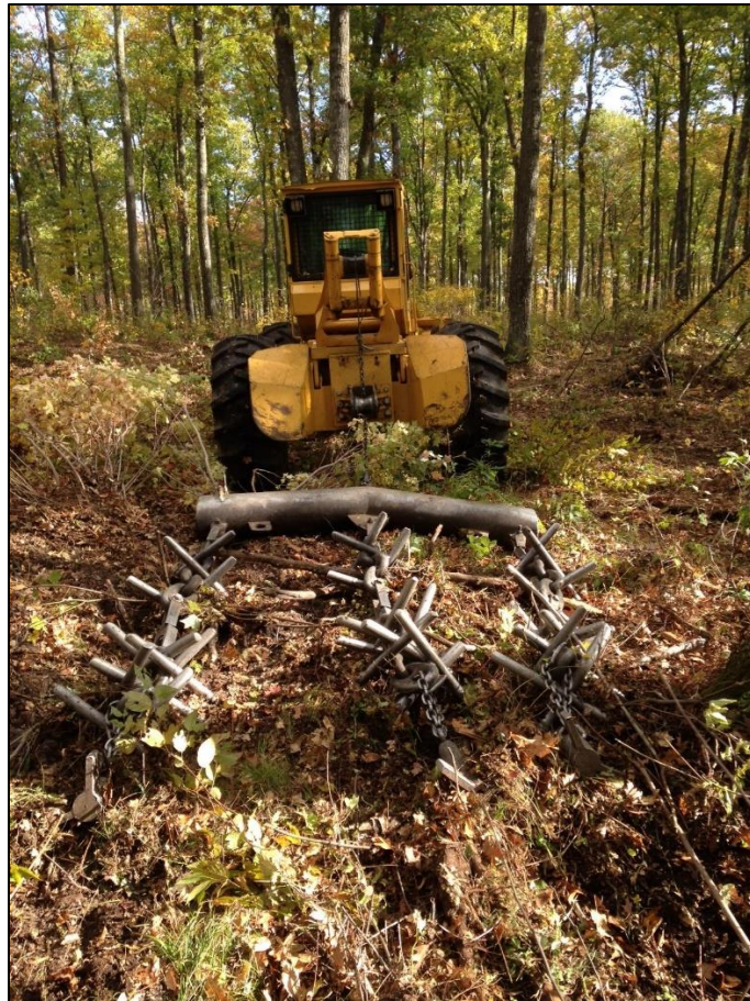
Anchor Chains Used For Understory Oak Scarification
