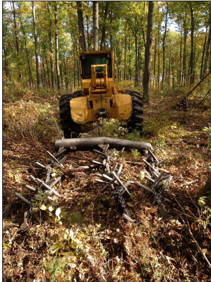
Anchor Chains Used For Understory Oak Scarification
